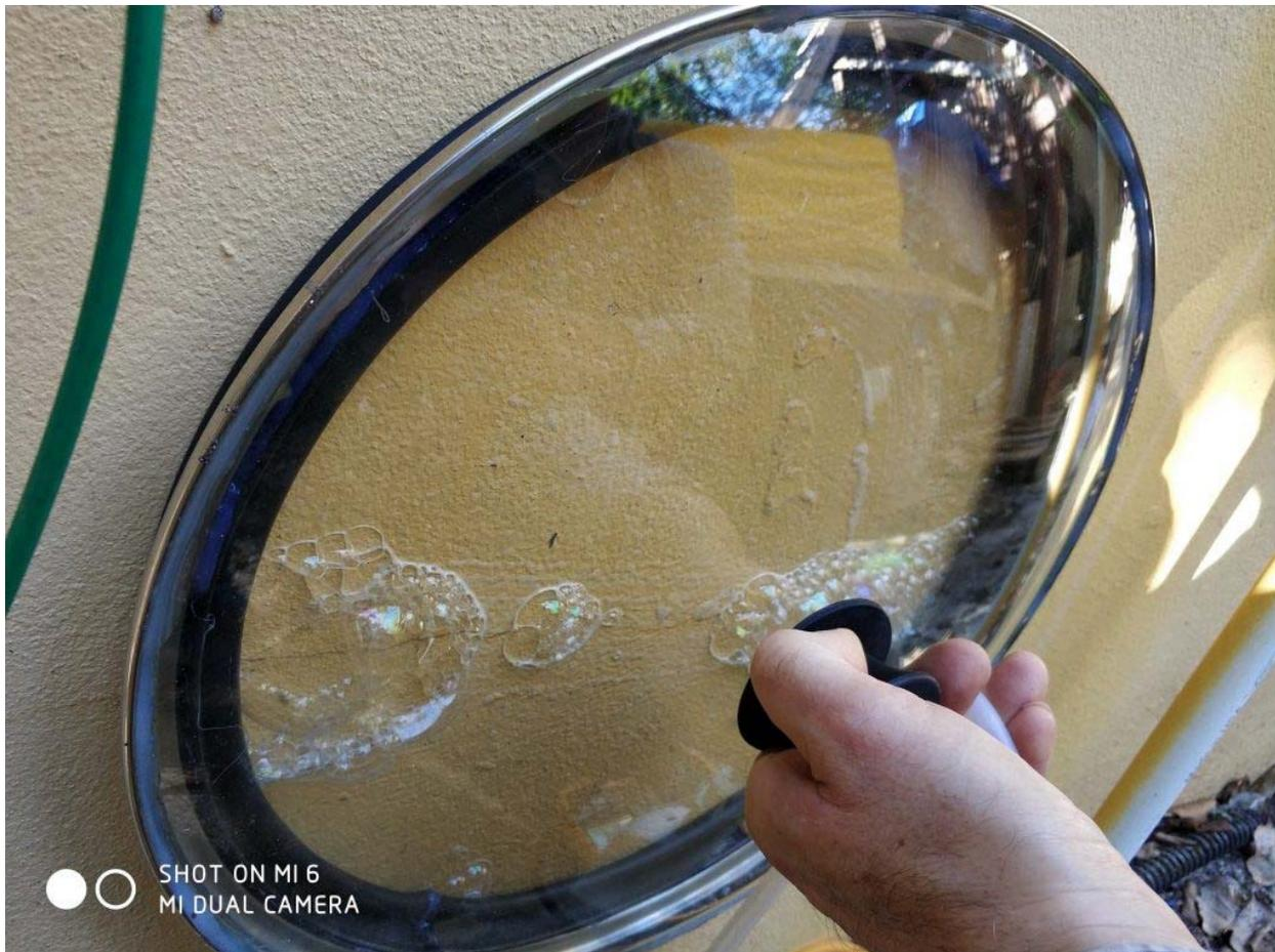
**Challenges.** The testing is used to assess only the typical flat surface, as opposed to e.g. material transitions. The most typical testing cases would be a liquid-applied WRB, and these are often installed on very rough surfaces, which may successfully resist sealing the chamber's perimeter, which in turn may need to be additionally sealed with some goop (e.g. *chewing gum*) or several additional hands pressing the perimeter gasket.
